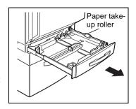
Press down on the paper-lifting plate until it locks into place.
